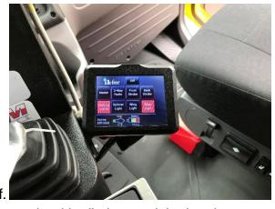
A CARB-compliant technology, Flex Systems comply with all city, municipal and state idling laws. All system functions are accessed via a small touch screen user interface located near the driver. Circuits controlled by the system are protected with a low-voltage disconnect. A timer on the touch screen displays cumulative runtime for the system making return-on-investment calculations easy for fleet managers.
